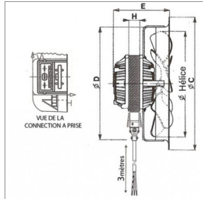
Côte d'encombrement : H = 25 mm / B = 290 mm / C = 305 mm / D = 264 mm / E = 115 mm
